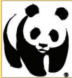
13. Adobe Streamline with its tolerance setting of 3 points produced 6 reasonably ACCURATE PATHS with 52 anchor points.
