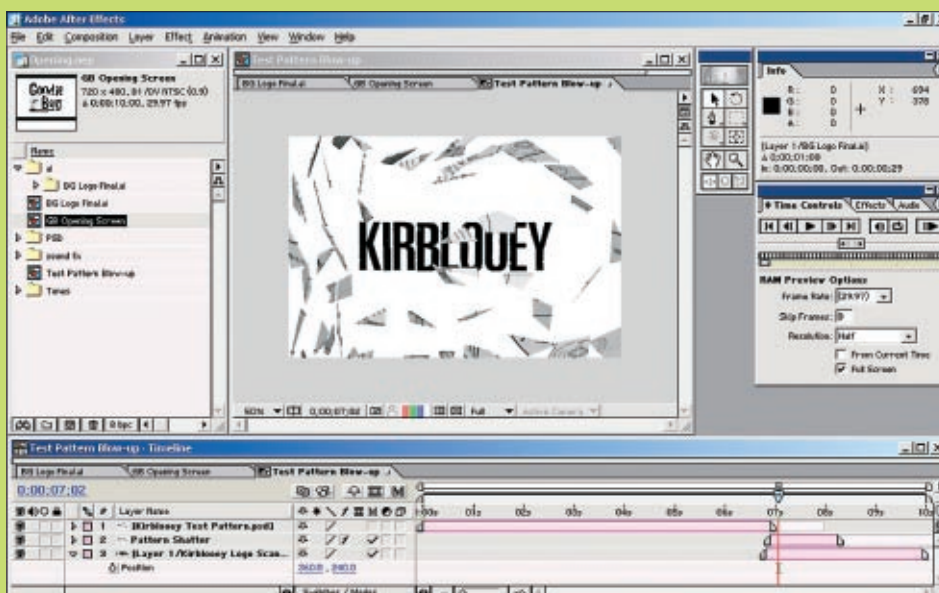
FIGURE 1. The Adobe After Effects WORKSPACE isn't quite like any other. In the upper left corner is the Project window. All imported footage (audio, video, stills), as well as the compositions you create, appear here. To the right of the Project window is the Composition window, where animations are constructed and previewed. In the Toolbox, note that the Pen and Marquee tools don't behave like they traditionally do – both are using for masking and won't create or select images. At the bottom of the screen is the Timeline. The position and length of footage within an animation's running time are represented by the coloured bars to the right of the layer name. Ghosted areas of the bar are trimmed segments of footage. Two toggle switches at the right of the layer name – Collapse Transformations (the star-shaped icon) and Quality (the diagonal line) – are used to preview at final render quality. There are three tabs in the Timeline and Composition windows, indicating three compositions are currently open. (A very unusual interface feature: there's actually a tiny, horizontal scroll bar at the top of the composition window.)
