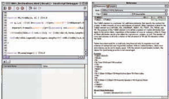
(left) The integrated JAVASCRIPT DEBUGGER checks your code for syntax errors, then runs with the browser to check for logical errors. (right) The O'REILLY CODE REFERENCE is a lookup system for JavaScript, HTML, and CSS. Click the Toolbar's Reference button and the panel gives a detailed description of your selected element.
