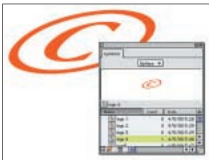
FreeHand's Flash-compatible SYMBOL LIBRARY allows the use of master elements across multiple pages — just drag new symbols into the Symbols panel and drag instances out.
