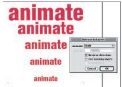
The RELEASE TO LAYERS feature creates animations and other motion effects without a timeline by translating layers into unique frames for Flash movies.
