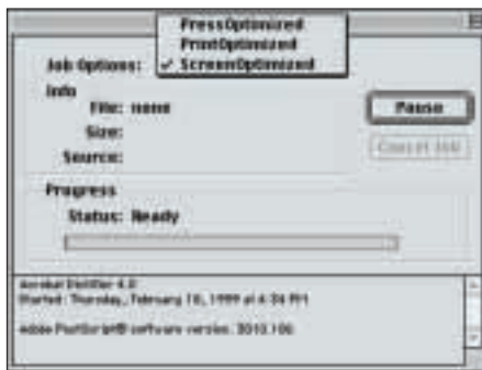
Acrobat Distiller now distills three primary types of PDF: for the screen, for printers, and for press.
