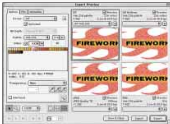
(above) Fireworks' Export Preview dialogue. Options, File and Animation panels let you experiment with file formats; compare the the output of color palettes and transparencies; and customize and save palettes, export presets and animation settings.
