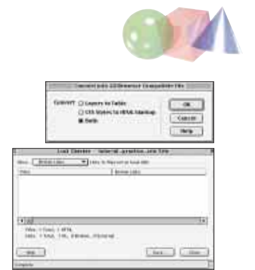
(top) The 'Convert to 3.0 Browser' command enables you to convert DHTML pages into pages compatible with 3.0 browsers. (bottom) The 'Check Browser' dialogue. This behavior automatically sends viewers to the page optimized for their particular browser.
