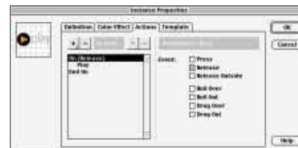
(top) Flash's toolbar, with the Arrow tool and modifiers selected; the Timeline, where you define the movie over time; the Stage, for creating and viewing the individual movie frames; and the Library, for managing symbols, bitmaps and sounds (bottom) The Instance Properties dialogue, with the Actions tab selected.
