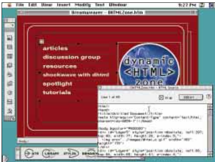
Dreamweaver's Document window and HTML inspector, plus the Object palette (left) and Launcher (bottom).
