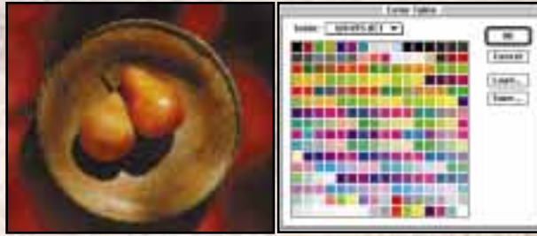
The adaptive palette looks the best because the colors are based on the content of the image. Paint Shop Pro calls this type of palette a Nearest Color palette. Photoshop calls it an adaptive palette.
