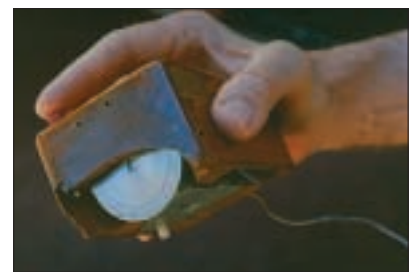
Engelbart's first mouse was constructed from a wooden block, a microswitch and two metal wheels, one running in each direction.
